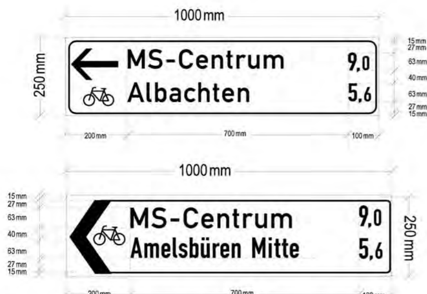
Dimensions of the NRW Bicycle road network signage
