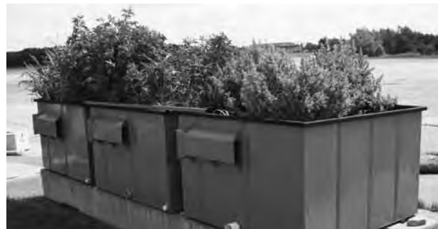
Bioretention pilot boxes installed at the Hydraulics, Sedimentation and Erosion Control Laboratory on TAMU Riverside Campus.
